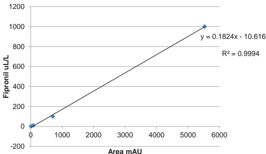
Fig. 2. Detector linearity of Agilent (Model 1200 series) high-performance liquid chromatograph equipped with an ultraviolet diode array detector;  $\lambda = 280$ , eluted by a Zorbax Eclipse XDB-C18 analytical 4.6 x 150 mm 5-micron column; limit of quantification was 0.01 $\mu$ l/liter.
